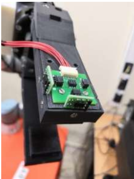
Figure 2. Realized prototype of the proximity sensors mounted on the sensorized finger used for testing.
