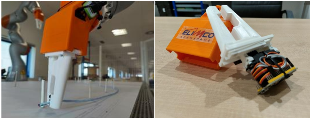
Figure 16: Self-manufactured grippers used at ELIMCO in early stages of the project
