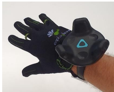
Figure 38. Sensors utilized to record the operator movements by the teaching by demonstration system: Dataglove and motion tracker.
