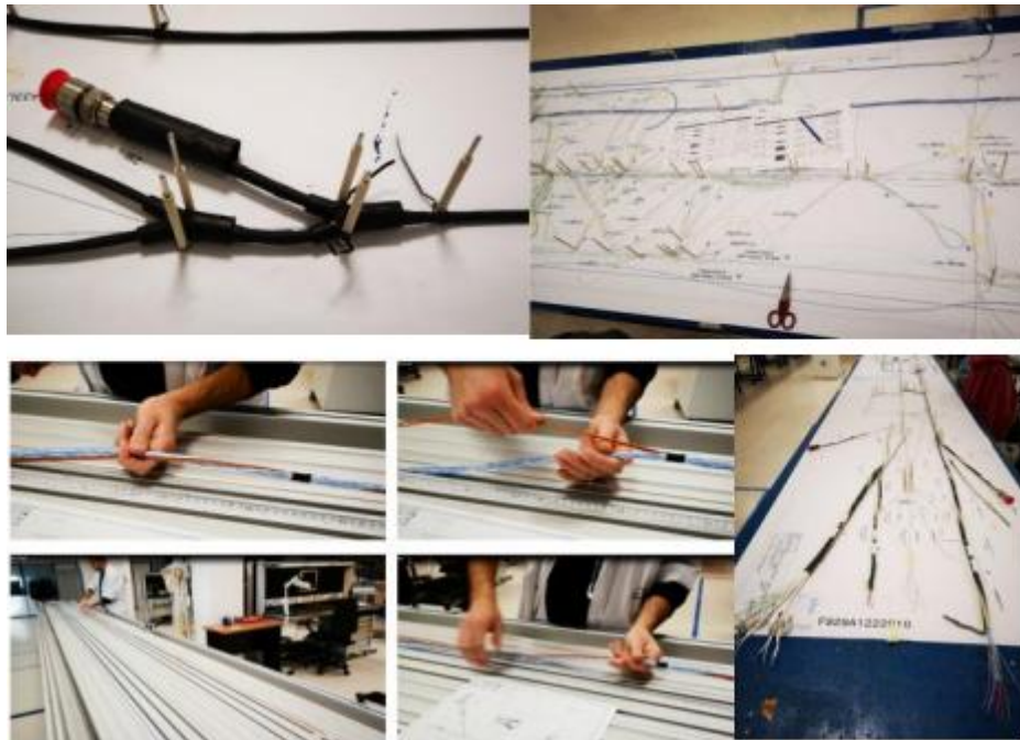
Figure 10: Manual wiring harness assembly
