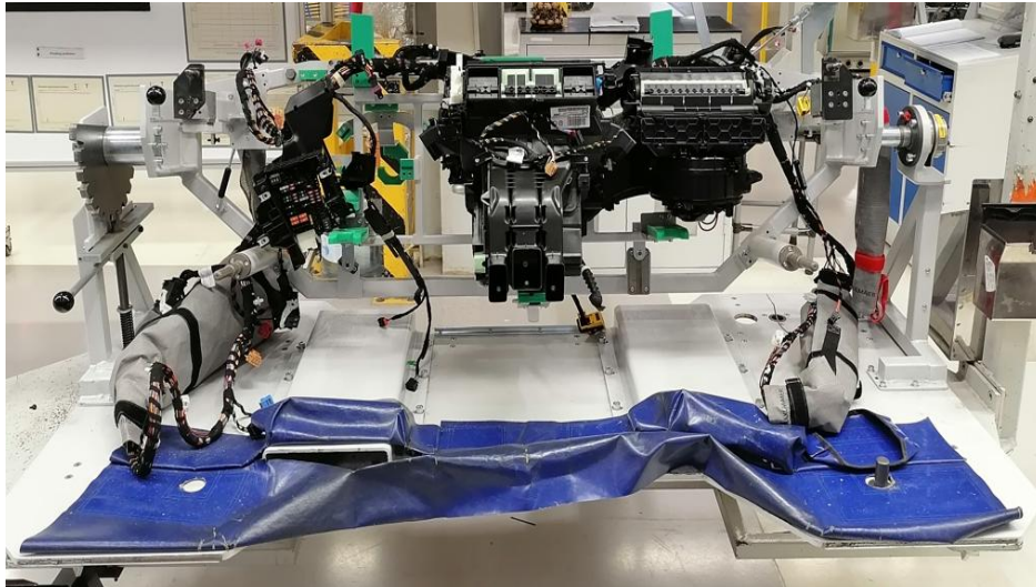
Figure 9 - view of the prepared cockpit wiring harness on the cockpit table
