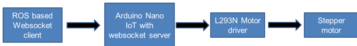
Figure 43. Communication for the taping gun actuation from ROS
