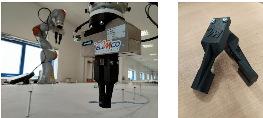
Figure 17: Schunk WSG50 grippers with extended fingers in ELIMCO use case
