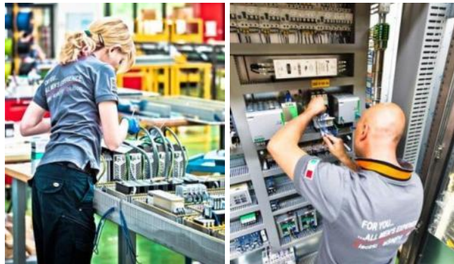
Figure 2 - Horizontal and vertical switchgear wiring
