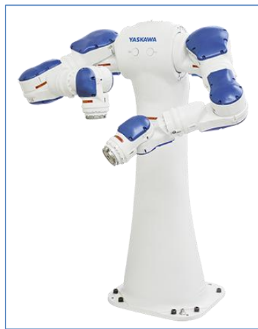
Figure 29. Yaskawa SDA10F Dual-arm manipulator
