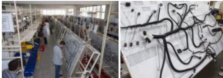
Figure 9. Wiring harnesses manufactured on pin boards
