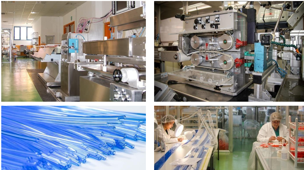
Figure 46 - Details of the ENKI production line, the extruder, the final product and the operators performing quality checks
