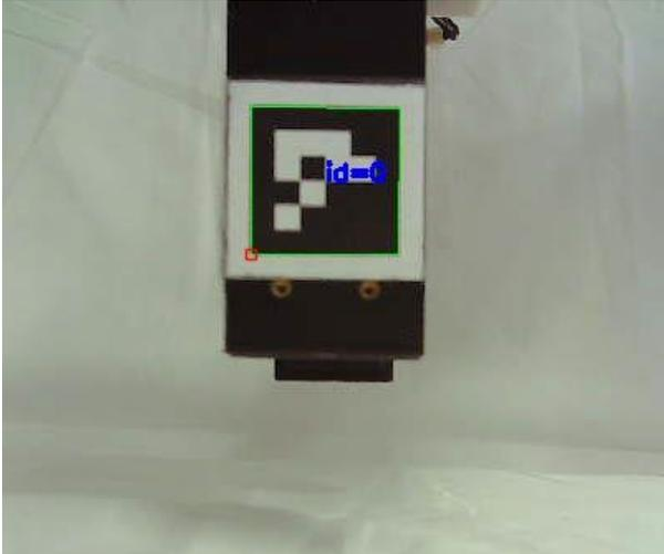
Figure 2: The marker placed on the finger used to detect the camera position.
