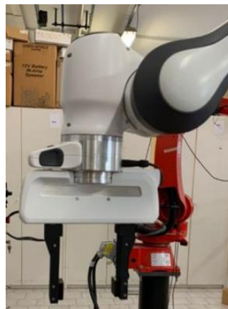
Figure 9 Sensorized fingers integrated in PANDA gripper
