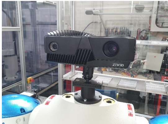
Figure 26. Zivid One camera mounted in the robot
