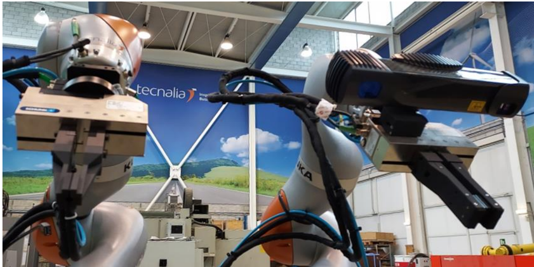
Figure 13. Schunk WSG50 grippers installed on robots for ELIMCO use case.
