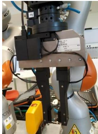
Figure 15 Sensorized fingers integrated in WSG-50 gripper
