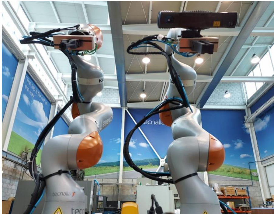
Figure 10. Kuka LBR iiwa robots for ELIMCO use case.
