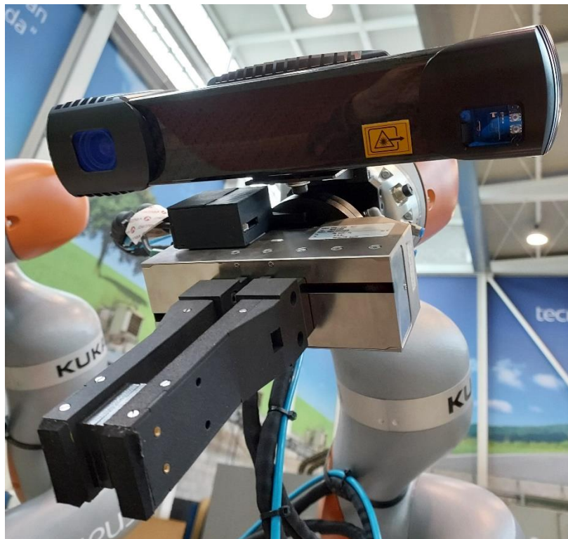
Figure 16. Photoneo MotionCam-3D camera mounted on robot in ELIMCO use case
