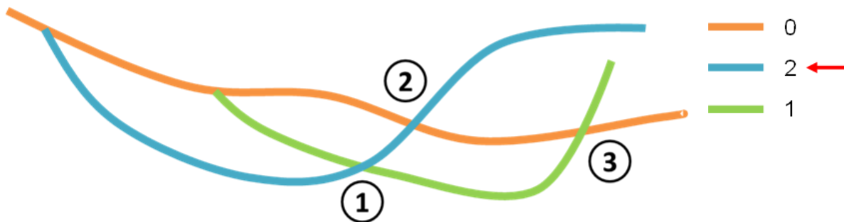
Figure 25: Left: Example scenario of an entangled wire harness. There are three sections (orange, blue and green) and three intersections. Right: Result after applying our WHDP algorithm to this scenario. The blue section has the highest counter value and thus should be manipulated first.
