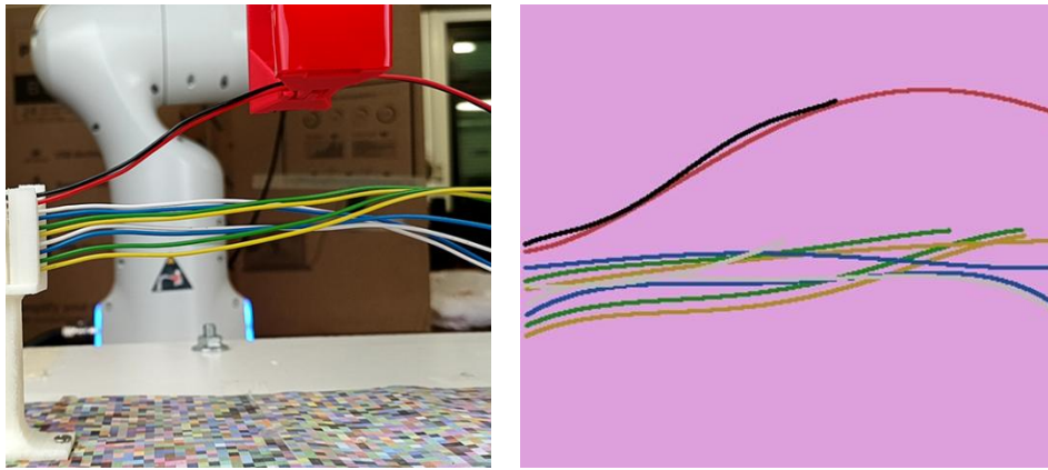
Figure 18: Cable physically separated by the manipulator
