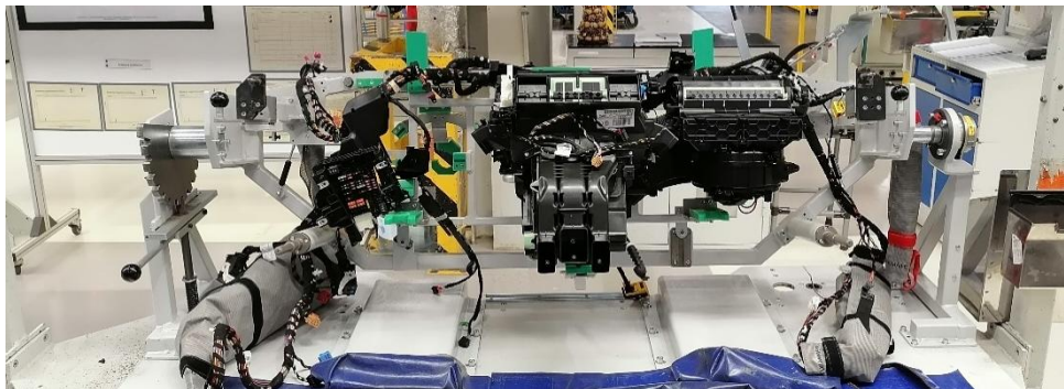
Figure 22: Overview of the cockpit with the wiring harness mounted. This is a desired state that has to be obtained after the manipulation.
