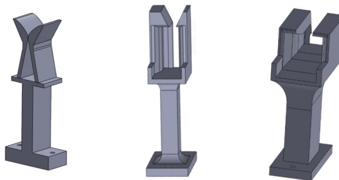
Figure 16 Design of the cable clips and connector holders.
