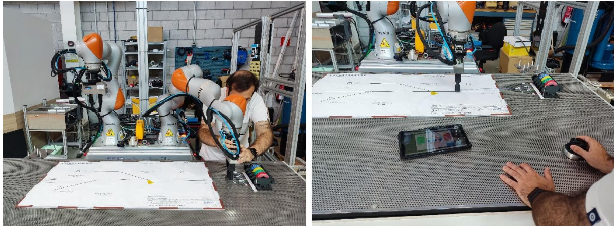
Figure 7 - Operator using kinesthetic and joystick-based teaching
